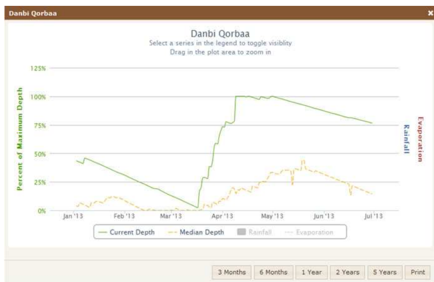
Fig. 5.9 Current information on the scaled water levels for Danbi Qorbaa (ETH-30) as shown on http://watermon.tamu.edu . The green line indicates scaled depth and the dashed orange line indicates long-term median depth
